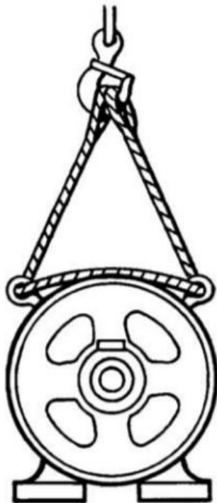
Bad practice – lifting on eyebolts from an angle reduces safe loads as much as 90%
